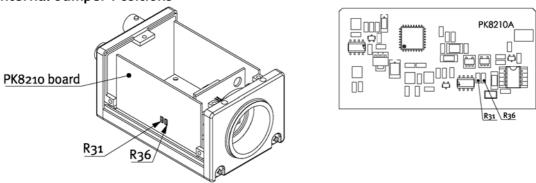
Fig. 20. Internal jumper positions
